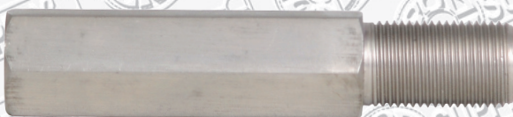
Female Adjuster 4.25" Length - 5/8-18 LH x 3/4-16 RH
